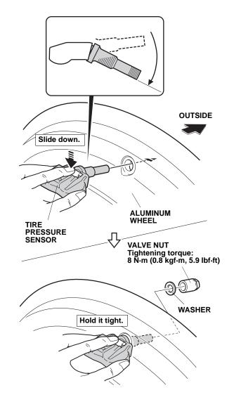
While holding the tire pressure sensor against the wheel, tighten the valve nut to the specified torque. Tightening torque: 8 N·m (0.8 kgf·m, 5.9 lbf·ft)
